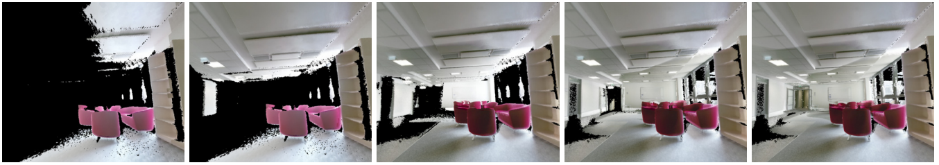
Fig. 8. Completion of scene model during capturing process: The images depict the scene model at different time steps. Depending on the regions that have been captured by the robot while moving through the scene, the captured 3D model of the environment gets more complete.
