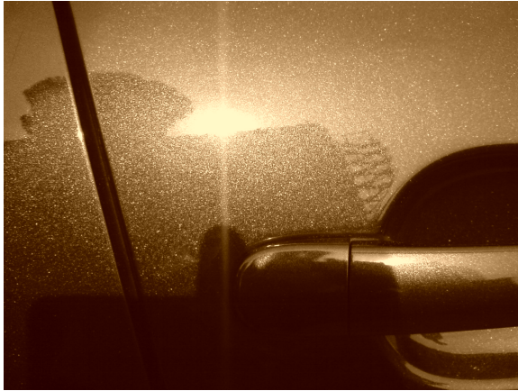
Figure 3: Photograph of a real car door part in bright sunlight. The depth effect and individual flakes remain visible even at several meters distance.
