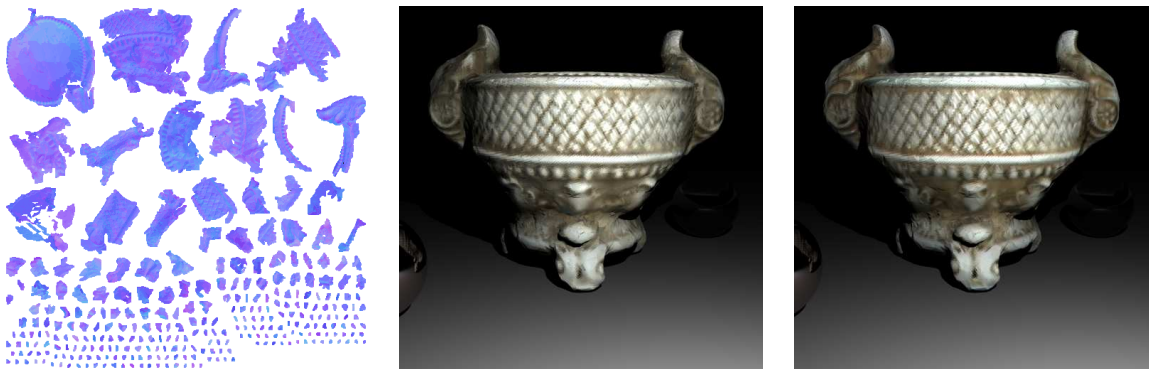
Figure 9: The precious vase data set. Left: the normal map computed by our algorithm. Middle: rendering from compressed representation (Local PCA - 22 MB). Right: rendering from losslessly compressed data (Lempel-Ziv - 2 GB)
