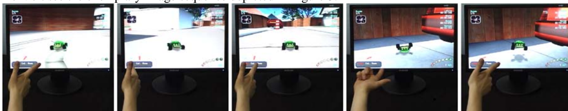
Figure 3: An exemplary image sequence of playing Re-Volt using our interface. Performed actions from left to right: turn right, turn left, drive straight, flip car, accelerate.
