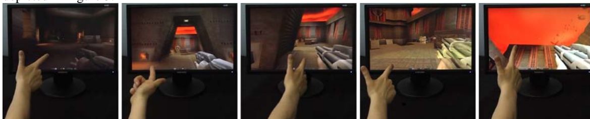
Figure 5: An exemplary image sequence of playing Quake II using our interface. Performed actions from left to right: turn right, change weapon, move straight, shoot, look up.
