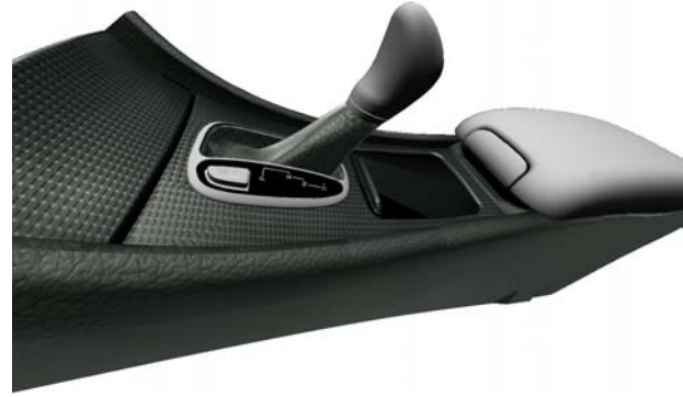
Fig. 3: Gear box model (courtesy of DaimlerChrysler) with parts covered with measured BTFs and other parts lit by a Phong model. While the reflection properties of the aluminium material appear much more realistic, the synthetic leather material nicely illustrates the enhanced depth impression generated by BTF rendering.
