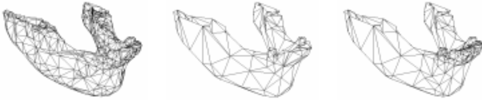
Fig. 5. On the left side the mesh of the mandible produced by the marching cube algorithm. In the middle a simplified mesh. On the right side mesh of the mandible is refined around the left tooth. The area of interest was defined interactively.
