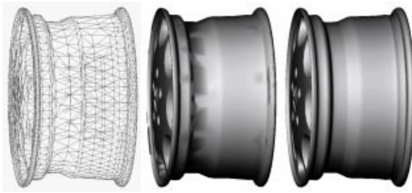
Fig. 2. The model of the rim in the middle is approximated by the level of detail shown in the picture on the left side. In areas where the direction of light is nearly perpendicular to the normals of the rim-surface already minimal changes of the normals lead to broad visible artifacts. The picture on the right side is generated using a view-dependent triangulation that take care of the illumination as described below. The artifacts disappear.
