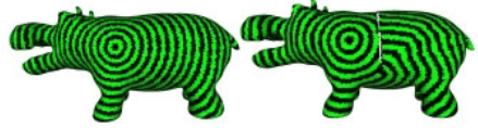
Figure 4: A gap in the hippo mesh on the right leads to unexpected distance values and therefore to non-intuitive editing results, whereas the left side hippo’s mesh is 2-manifold and the geodesic distance field behaves as supposed.
