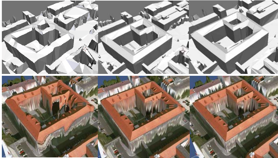
Fig. 2: Simplification results. Left column: unconstrained, 4m threshold. Middle column: constrained, 4m threshold. Right column: constrained, 32m threshold. The upper row shows the shaded TIN whereas the lower row shows a rendering textured with full 12.5cm resolution.
