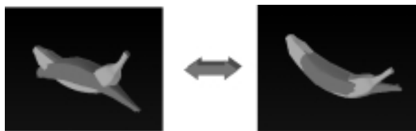
Figure 3. Both depicted configurations have the same principal axes and eigenvalues – further computations are needed to align the objects properly.
