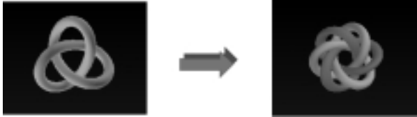
Figure 4. The depicted object has a completely symmetrical mass distribution around the z axis rectangular to the image plane. Therefore an infinite number of valid principal axes exist – an extended approach is called for.
