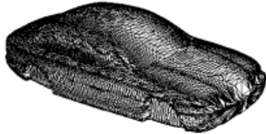
Figure 14: Reconstruction of a BMW from about 100 contour slices. The slices were generated by a laser range scanner. In the first step the scanner data was converted into polygons. In the second step, the polygons were simplified and then the actual reconstruction took place. In this example picture after the reconstruction step no further simplification was performed. Data by BMW AG München.
