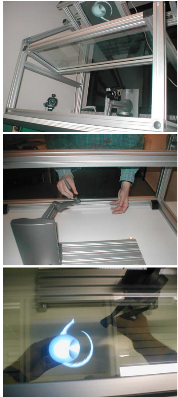
Figure 2: The MEW. Top: Total. Middle: Edit session from behind. Bottom: A possible augmented workspace with a virtual object (simulation).
