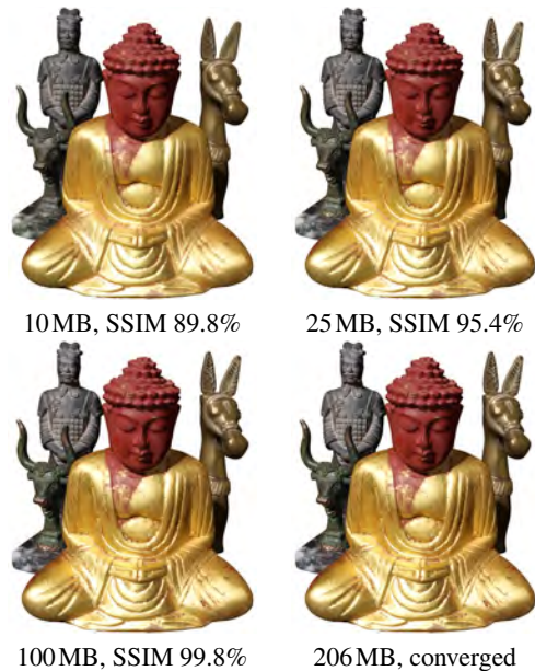
Figure 5: Rendering quality after streaming different amounts of data over the network. The SSIM values predict the perceptual similarity between the images and are computed with respect to the converged version.
