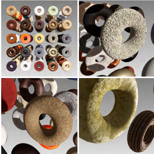
Figure 2: Screenshots of a fly-through animation in a virtual scene with 100 different measured BTF material having a size of 512 \times 512 texels. The scene renders with 35 FPS at 1280 \times 720 pixel on a NVIDIA GeForce GTX 680 GPU. While the total amount of the factorized BTF data is 6.2GB, the memory footprint on the GPU using BSVTFs is 1.7GB.
