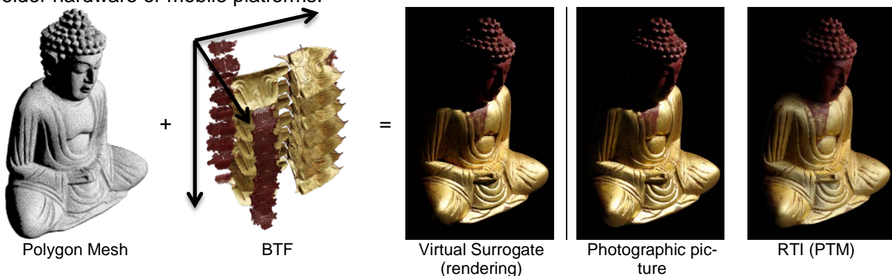
Figure 5: the virtual surrogate consists of a polygon mesh and the BTF. The rendering of the virtual surrogate reproduces the appearance to a photographic picture from the measurement. An RTI created from the same measurement data fails to reproduce effects at the macroscale, e.g. the shadow of the head and hands, and at the microscale, e.g. the highlights of the red paint and gold.
