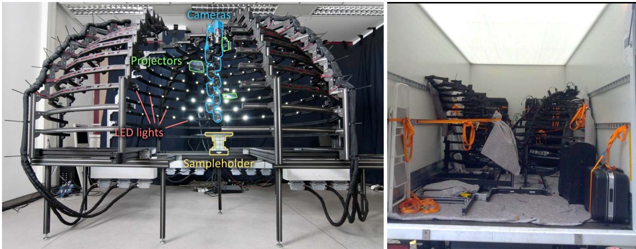
Figure 4: the proposed multiview/multilight dome setup. Left: fully assembled, the front-left quarter is slid open to give a better view on the components. Right: the dome is disassembled and packed in a single transport van.
